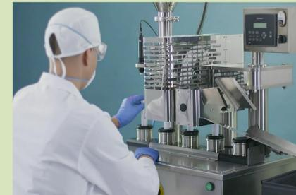
Figure 2: Semi-automatic aluminium tube filling and crimping machine
