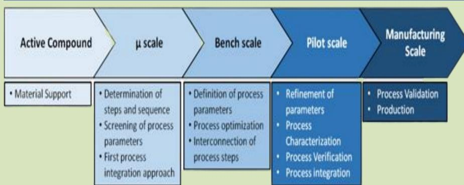
Figure 1: State of the art process of up-scaling
